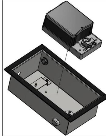
3. Connect the valve assembly to the base of the rain hood, apply the washers and then tighten the nuts onto the actuator adaptor.
