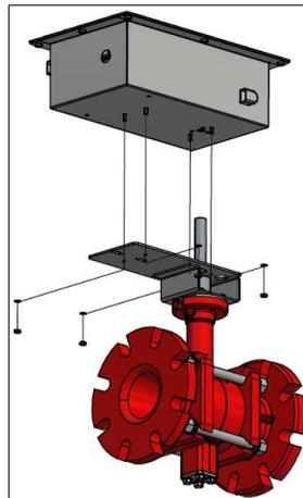
4. Wire the actuator according to the local electrical code. Ensure that UL listed electrical fittings for NEMA type 3 conditions are used for the hole provided.
